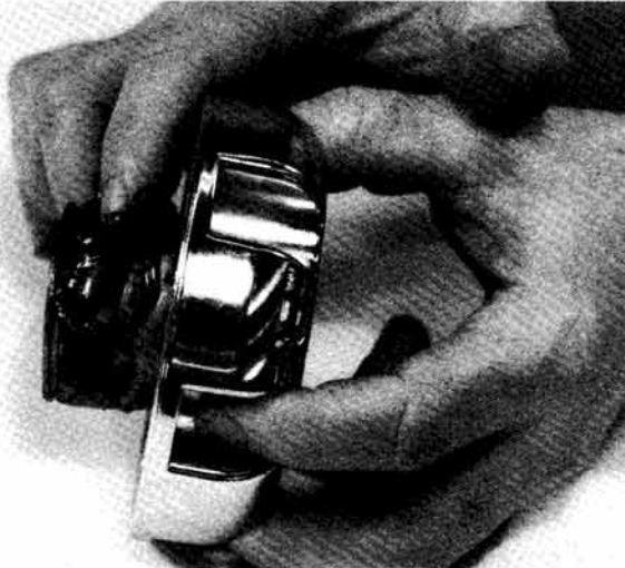
Figure 5 1001-15 Turn actuator knob to LOCK position. Apply a small amount of Moly XL hi-speed grease to both grooves of the cam as shown.
